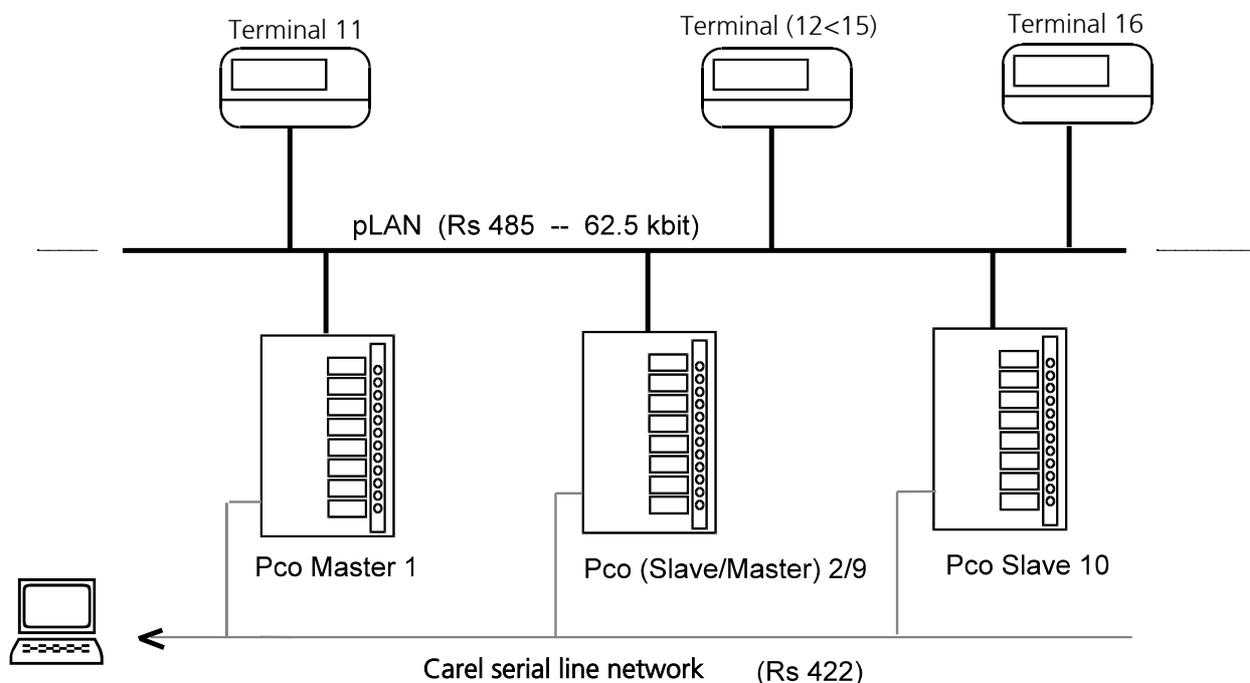
The Master boards can have the address 1, 3, 5, 7 or 9, and the corresponding Slave boards must be given the address 2, 4, 6, 8 or 10.
